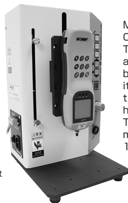
MODEL-1308U Capacity / 1000N The gage mounting part is moved up and down electrically. The power supply is a multi power supply of 100 V to 240 V.
