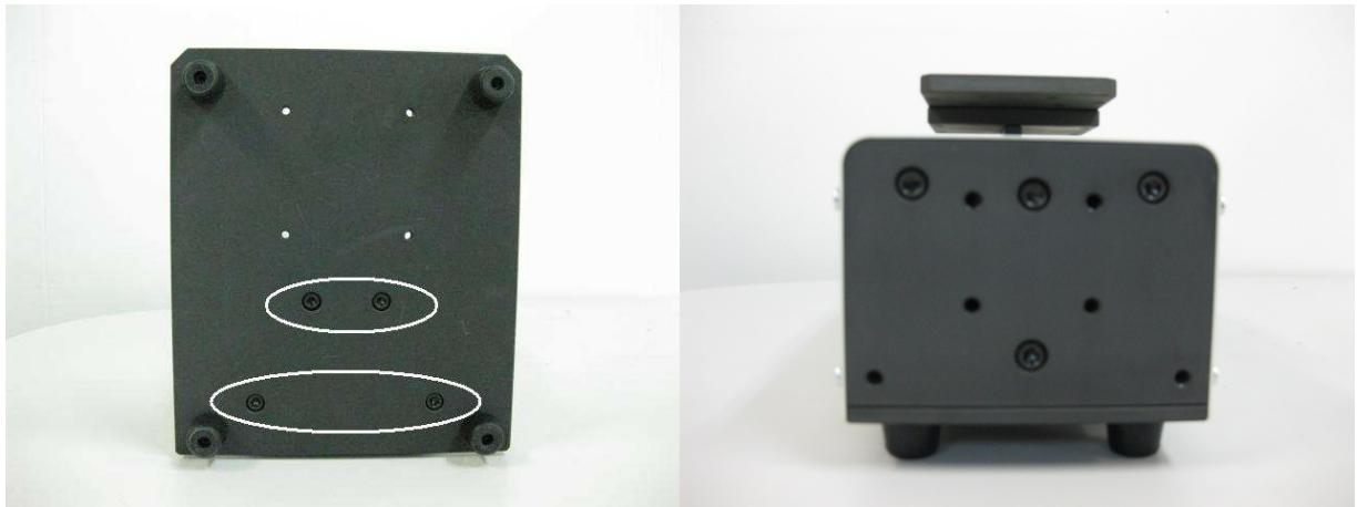
2. Fix the L plate for the horizontal type with the large head screws supplied with the test stand.
