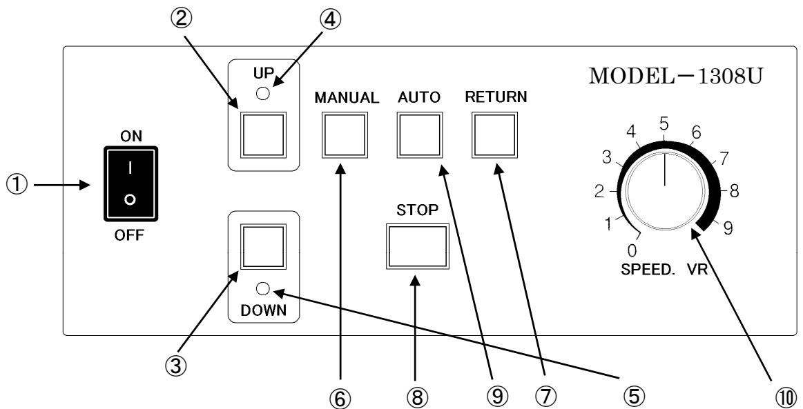
① Power switch: Press the ON-side position of this switch to turn on power. Press the OFF side to turn off power. The test stand will not operate when it is turned off.
