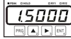
Press the **PRG** key twice to set the CAL mode. Operate the **▲** key/**▶** key to enter a value. To register a new load cell, check the rated output shown on the load cell test report.
