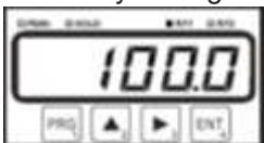
Press the **PRG** key 5 to 6 (7 to 8) times to set the RELAY 1 (2) H/L input mode. Set the RY1 (2) H (upper limit) High and set RY1 (2) L (lower limit) Low.
