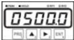
Press the **PRG** key 3 times to set the SCALE (rated capacity) mode. Operate the **▲** key/**▶** key to enter a value. To register a new load cell, check the rated capacity shown on the load cell test report.
