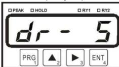
Press the **PRG** key 10 times to set the display speed mode. Operate the **▲** key to select a speed; 1, 2, 5, 10 and 15 times per second.
