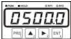
Press the **PRG** key 4 times to set the AUTO CAL mode. Apply a test load (weight, etc.) on the load cell and enter the applied test load by operating the **▲** key/**▶** key. When the **ENT** key is pressed, force calibration can be conducted automatically.
