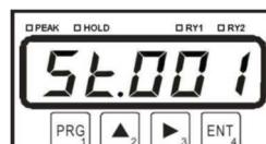
Press the **PRG** key 11 times to enter the display step set mode. Operate the **▲** key/**▶** key to change the value. A value can be set in a range of 0 to 255. The last digit of the value will change at the set value.
